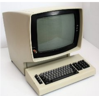
IBM 3270 terminal, used to access mainframes using TSO (Time Sharing Option).
